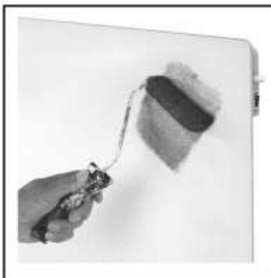
What is unique about the E-convect, is that it can be painted. You can paint the E-convect in any color you wish, with any water resistant paint. Do not paint the box with the switch and remove the plug from the socket before you start painting. Allow the panel to dry before using it again!
