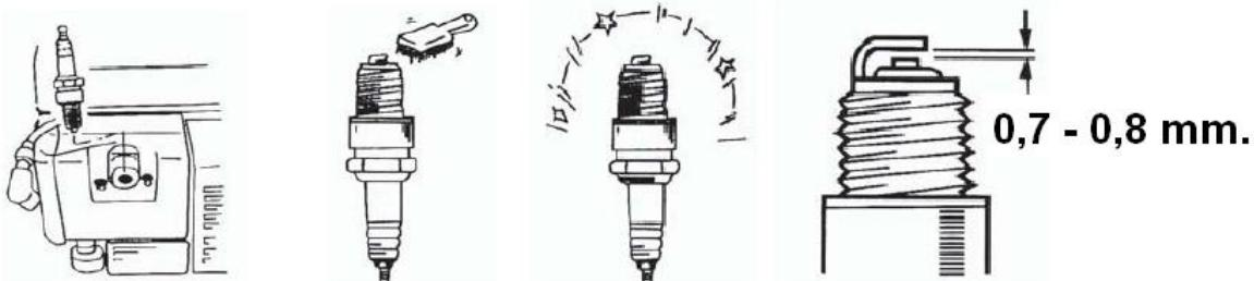
Check the spark plug after 50 working hours. Remove any carbon build-up, check to ensure the spark plug is not discoloured and, if necessary, set the opening (0.7 to 0.8 mm.), or replace the spark plug with another of the same type.
