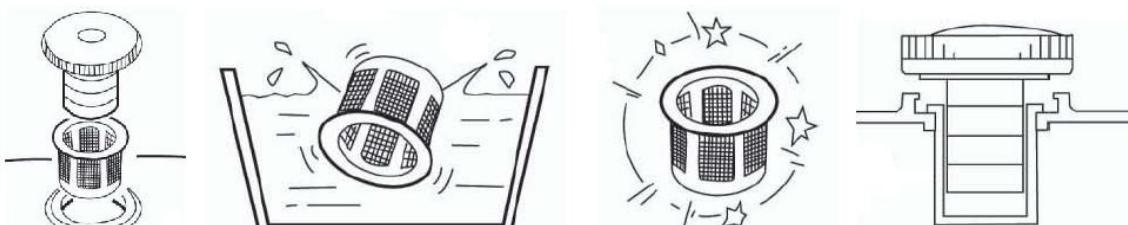
Clean the fuel filter after every 150 working hours/3 months (whichever comes first); the fuel filter is found in the filling opening, under the cap. Take the filter out of the opening, clean it in a little clean petrol, dry and then replace. A damaged or worn fuel filter must be replaced. Never run the generator without the fuel filter!
